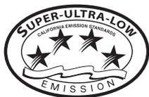
Sterndrive and inboard marine engine powered boats meeting CARB's exhaust emission standards are required to display the four-star label on the outside of the hull above the waterline. Outboard and personal watercraft marine engines may also comply with these standards.
