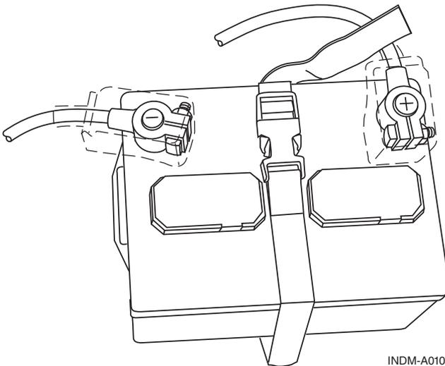
**Figure 3.4 – Battery Connections**
